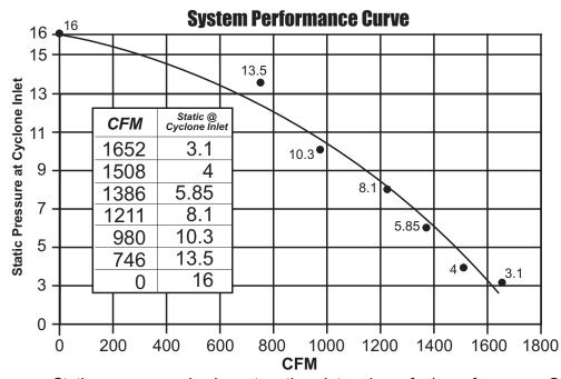
Static pressure and volume together determine a fan's performance. Several factors, such as layout of ductwork and diameter of openings, can affect a fan's performance.
