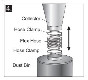
Attach the ductwork from the woodworking machines to the inlet of the collector.
