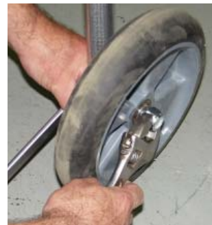
Figure 13 - Tighten wheel nuts
