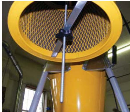
Figure 32 - Attach rod & silencer w/ thumb nut.
