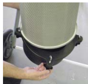
Figure 35 - Attach dust bin with J-hooks
