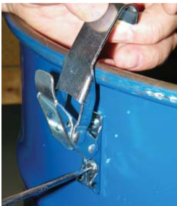
Figure 2. Dust drum latches and hardware.
