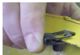
Figure 23 - Attach U - spring nut
