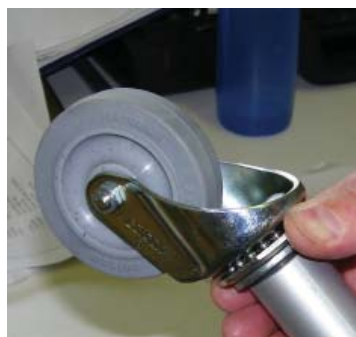
Figure 17 - Tighten Nut on caster.
