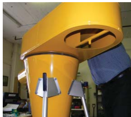
Figure 22 - Attach Blower housing
