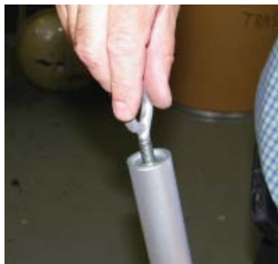
Figure 9 - Screw eyebolts into threaded inserts.
