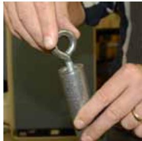
2. Before you attach the legs to the bracket, you must put end caps in the back legs. Screw an eye bolt into the end cap as shown above. Leave about 1/4" of thread showing. Then gently with a hammer, hit the eye bolt to force the end cap evenly into the leg end until it is flush and centered. The axle goes through the back leg eye bolts.
