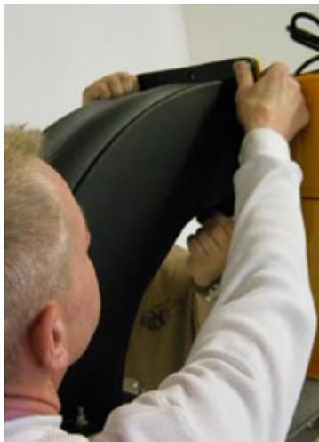
13. Use the (7) 3/8" hex head bolts (AFS015100), (14) washers (AFW190000) and (7) whiz nuts (AFT000004) to attach the plenum are in the kit hardware. Use the following order: bolt / washer / outlet / plenum / washer / whiz nut. /
