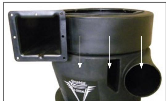
**6. Carefully lift fan housing to top of barrel section keeping gasket side up. Carefully line up the holes in fan housing with the holes in the barrel section, keeping in mind the direction you want your outlet to face. Then attach using provided (8) 5/16" flange bolts (AFB155155). Do not use over 17 ft. lbs. of torque. You will need a sturdy step ladder for this.**
