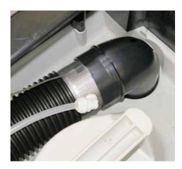
The photos above show a grounding solution if you are using a Festool mini extractor. You will need to use an elbow to attach the hose to the inlet. You need to tape the elbow with the metal tape first as shown on previous page before you attach it to the hose and metal connector. You also need to tape the pre-installed grounding wire from the metal connector to the top of the Festool as shown at top left.
