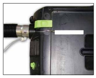
3. Take the braided wire and run it over the top of the Festool Extractor as shown left and then tape the wire down securely with a 4" piece of metal tape so it will contact the electrically conductive Oneida Dust Bin when it is attached to the extractor.
