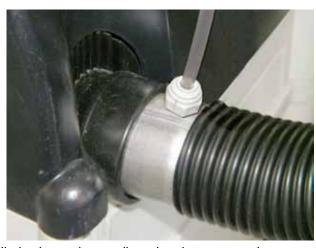
2. Attach hose to the smaller end of the metal connector with pre-installed valve and grounding wire, then connect hose to the vacuum inlet as shown in picture above right.
